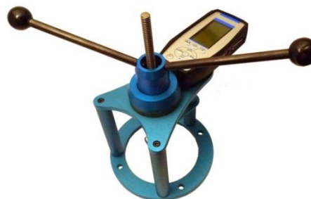
Figure 20: Pull tester for adhesion testing. (Photo courtesy of Com-Ten)
