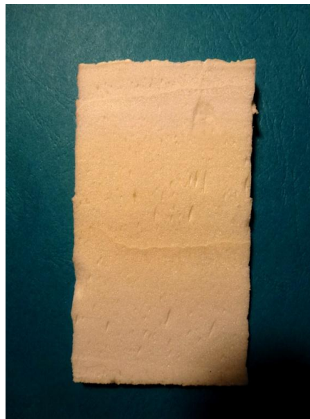
Figure 13: This specimen was cleanly sliced from a cylindrical core sample.
