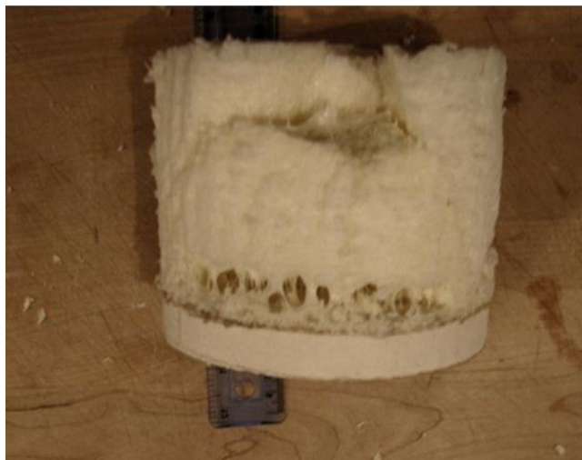
Figure 18: Example of open, irregular cells. (Photo courtesy of the Spray Polyurethane Foam Alliance)
