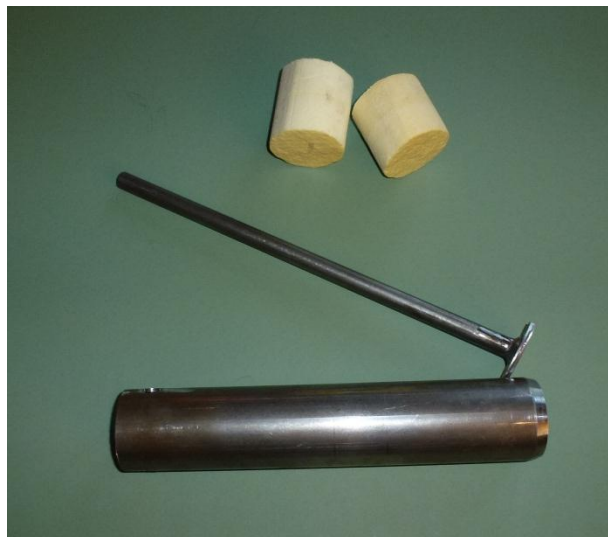
Figure 11: Coring tool with handle/pusher and plugs.
