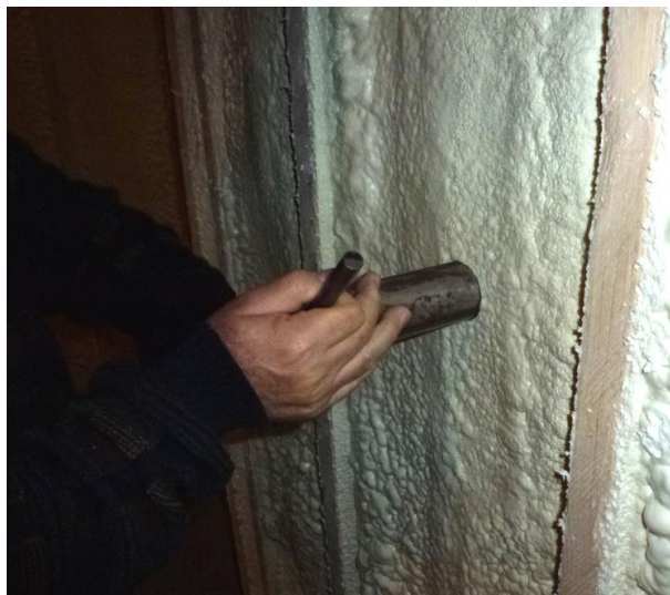
Figure 12: Using the coring tool to extract a core sample.
